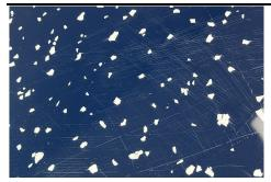
Superficial scratches and scuffs can happen for many reasons including (but not limited to) dragging objects, sliding objects, or moving objects that make contact with the topcoat of the flooring system. Examine damaged area by feeling for the depth of the scratch or scuff with your fingernail.
