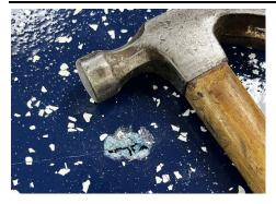
Impact damage can occur when sharp or heavy objects are dropped on the flooring. There are also different types of impact damages including the type that damages only a coating to a substrate, damage of coating to underlayment (but underlayment adhesion to substrate is still intact), and impact damage of an entirely underlayment system with the substrate. Below are steps to take when there has been impact damage that created cracks or delamination for these various types of situations.
