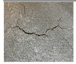
Ships often experience harsh environmental conditions such as large swells, high winds, and extreme temperature fluctuations. These types of conditions typically result in ship movements such as roll, pitch, yaw, and flex. During these situations, a deck can twist and flex to a point where the deck will create a crack. These cracks need to be addressed as soon as possible to prevent water intrusion and eventual deck failure.
